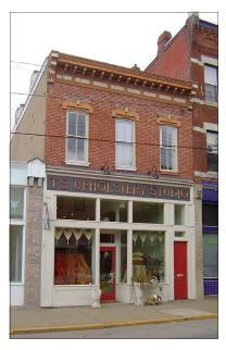
Figure 34. Signboard with individual letters and gooseneck lighting
